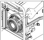
NOTICE Do not allow the starter grip to snap back against the engine. Return it gently to prevent damage to the starter or housing.
