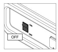
3) Turn the fuel valve to the "OFF" position.
